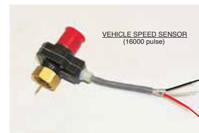
Typical 3 wire Autometer 5291 VSS connection
